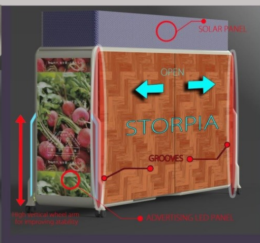
Shutter open inspired by traditional Japanese doors and sink down in grooves set in chassis of the STORPIA
